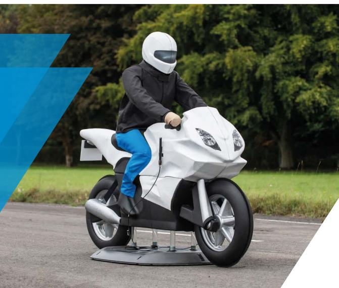
The Soft Motorcycle 360 from DRI is a durable and realistic surrogate motorcycle target that is stable at speeds of up to 80km/h. Its rotating wheels and realistic shape mean that it is reliably recognised by vehicle sensor systems including cameras, radar and lidar.
