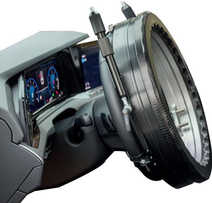
The Halo robot is a direct-drive hollow centre steering robot that enables a wide range of steering inputs to be applied with high precision and repeatability, so that high quality data can be captured.
