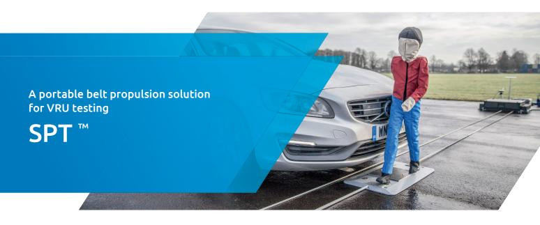
The Soft Pedestrian Target (SPT) system is a portable belt propulsion mechanism which uses our patented Synchro™ technology to accurately and consistently play out NCAP and custom-made test scenarios.
