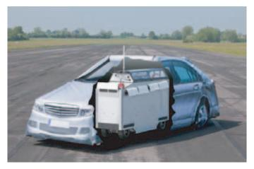
Fig 5: Soft Crash Test Vehicle
