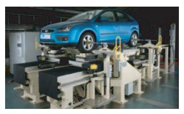
Fig 1: Suspension Parameter Measurement Machine
