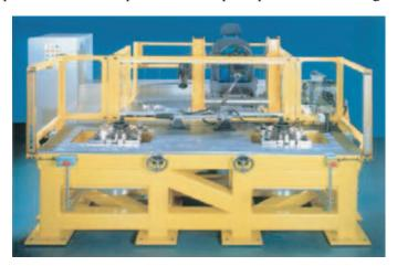
Fig 2: Steering System Test Machine
