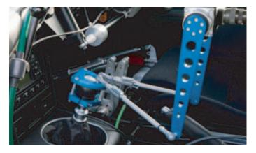
Fig 3: Gear Shift Robot
