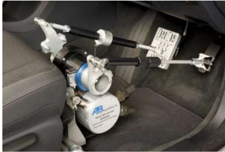
CBAR (combined brake and accelerator robot)
