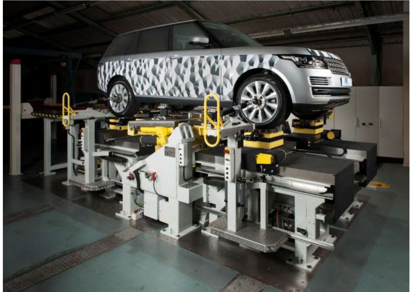
SPMM5000 used for suspension characterisation
