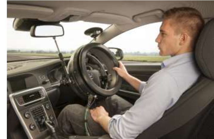
Patented SR60 Torus steering robot
