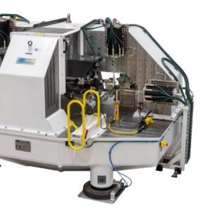
The ANVH 250 is a sophisticated axle-level test machine that accurately measures noise, vibration, and harshness (NVH) transmission through a suspension system into a vehicle body.
