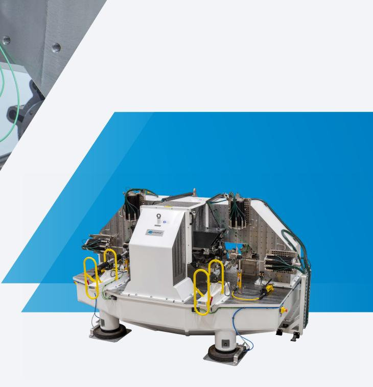
The ANVH 250 can apply sinusoidal, random input and road load data displacements to the suspension system. Displacements can be applied to the wheel hubs in the vertical (Z), longitudinal (X) or lateral (Y) directions. The paired displacements at the hubs can be in-phase, anti-phase or single-sided.
