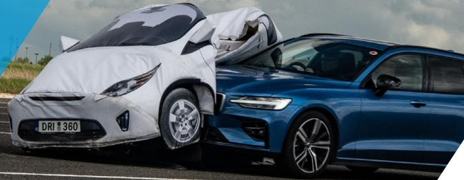
The GST 120 is the most capable surrogate vehicle system currently available for testing vehicle Advanced Driver Assistance Systems (ADAS). With a top speed of 120km/h, GST 120 is the only product on the market capable of testing highway assist and drive pilot systems at realistic highway speeds.
