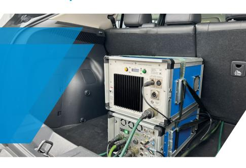
The Independent Power Pack is compatible with our range of driving robots and can be installed quickly without connecting to a vehicle's power system.
