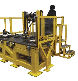
The SSTM is an advanced steering system test machine that enables characterisation, mechanical hardware-in-the-loop (mHiL) and driver-in-the-loop (DiL) activities to be completed on hydraulic, EPAS and drive-by-wire steering systems.
