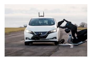
The Soft Scooter 360 has been developed in response to the growing global demand for scooters and e-scooters. The target meets the ISO/WD 19206-5 standard and is compatible with C-NCAP 2021 protocols. The test scenarios it can be used for includes:
