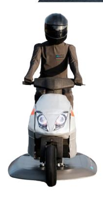
The Soft Scooter 360 is a highly realistic and cost-effective surrogate scooter target that is stable up to speeds of 60 km/h. Its realistic shape, speed-matched rotating wheels and photorealistic vinyl skin increases recognition and detection by vehicle sensor systems, including camera, radar and lidar.
