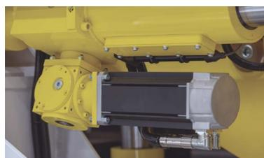
Servo-electric linear actuators
