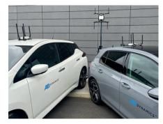
TrackFi PowerMesh is a premium dual band wireless mesh network, capable of creating secure scalable wireless networks to provide low latency high bandwidth data transfer between multiple vehicles. Part of AB Dynamics track testing offering, TrackFi PowerMesh supports the communication needs for Driverless Test Systems, synchronisation testing and real-time monitoring of motion pack data.
