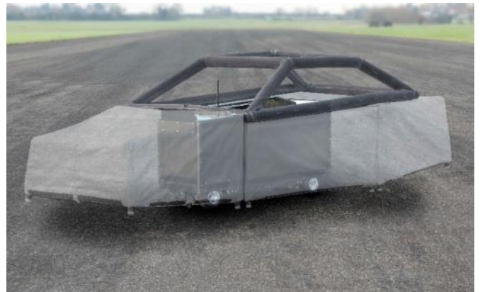
SCT showing the central drive box
