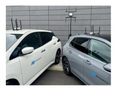
TrackFi PowerMesh is a premium dual band wireless mesh network, capable of creating secure scalable wireless networks to provide low latency high bandwidth data transfer between multiple vehicles. Part of AB Dynamics track testing offering, TrackFi PowerMesh supports the communication needs for Driverless Test Systems, synchronisation testing and real-time monitoring of motion pack data.
