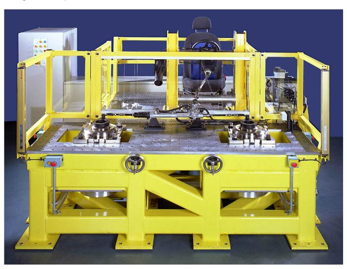
The frame of the machine allows the vehicle s steering column and steering wheel to be mounted so that manual inputs can be applied to the system (a seat is provided for the driver), and steering feedback to be measured. Optionally, the machine can be interfaced with ABD s SR30, SR60 or SR80 Steering Robots, to provide controlled position or torque inputs to the steering column.
