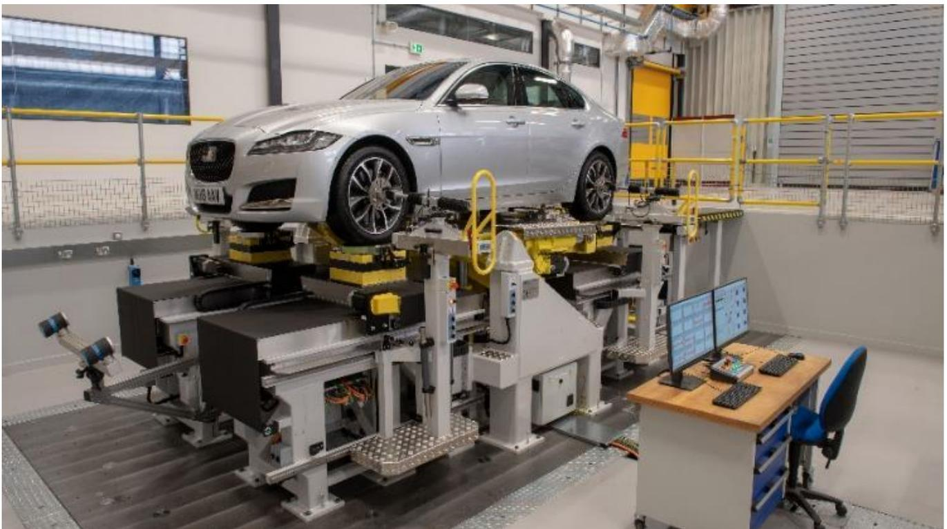
The system supports the EtherCAT fieldbus protocol, allowing it enough performance to run the motion control at a PWM frequency of 4kHz, previously this was 2kHz.
