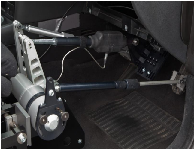
Under-seat pedal actuators (throttle, brake and clutch)
